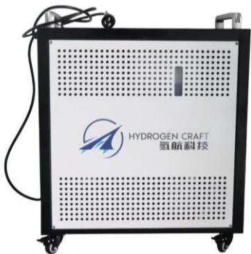
This 0,3 Nm<sup>3</sup>/h PEM hydrogen generator uses renewable energy (solar or wind, even with unstable energy supply) and purified water (conductivity  $\leq 0,1$  mS/m @25°C) to produce clean, green hydrogen through electrochemical reaction.
