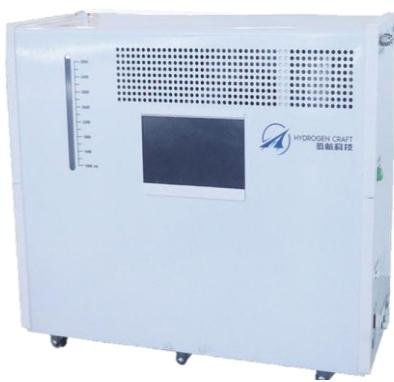
This AEM electrolyser is fully integrated, ready to produce, and it is used for electrolyzing water to produce high purity hydrogen at atmospheric pressure up to 3MPa. It has the features of simple interface, user-friendly, safe and reliable, while it can operate with constant hydrogen flow and constant pressure, and provide stable pressure or flow of hydrogen, without hazardous waste products.
